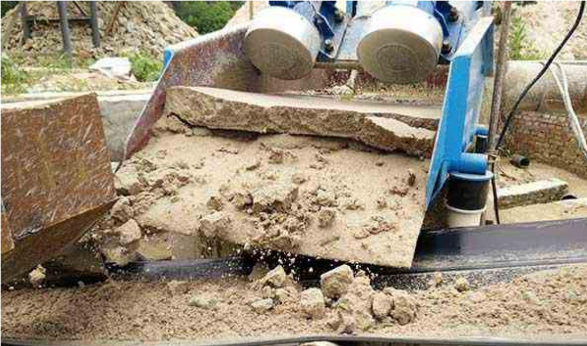
Dewatering screen is a common tool, which can not only used in sand processing plant, also can used in mine, ores, clay, slurry, concrete mixing plant, etc. And the feed to dewatering screen can come from a variety of sources, include material washing machine, cyclones, density classifiers, and even directly from classifying tanks.
