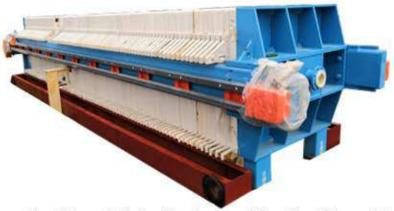
The plate and frame filter press is arranged in parallel with the filter plate and filter frame with the filtrate passage. And a filter cloth is sandwiched and pressed between each filter plate and filter frame to form a filter chamber. The sludge is flowed from the feed inlet, the water is discharged from the filtrate outlet through the filter plate, and the mud cake is accumulated on
