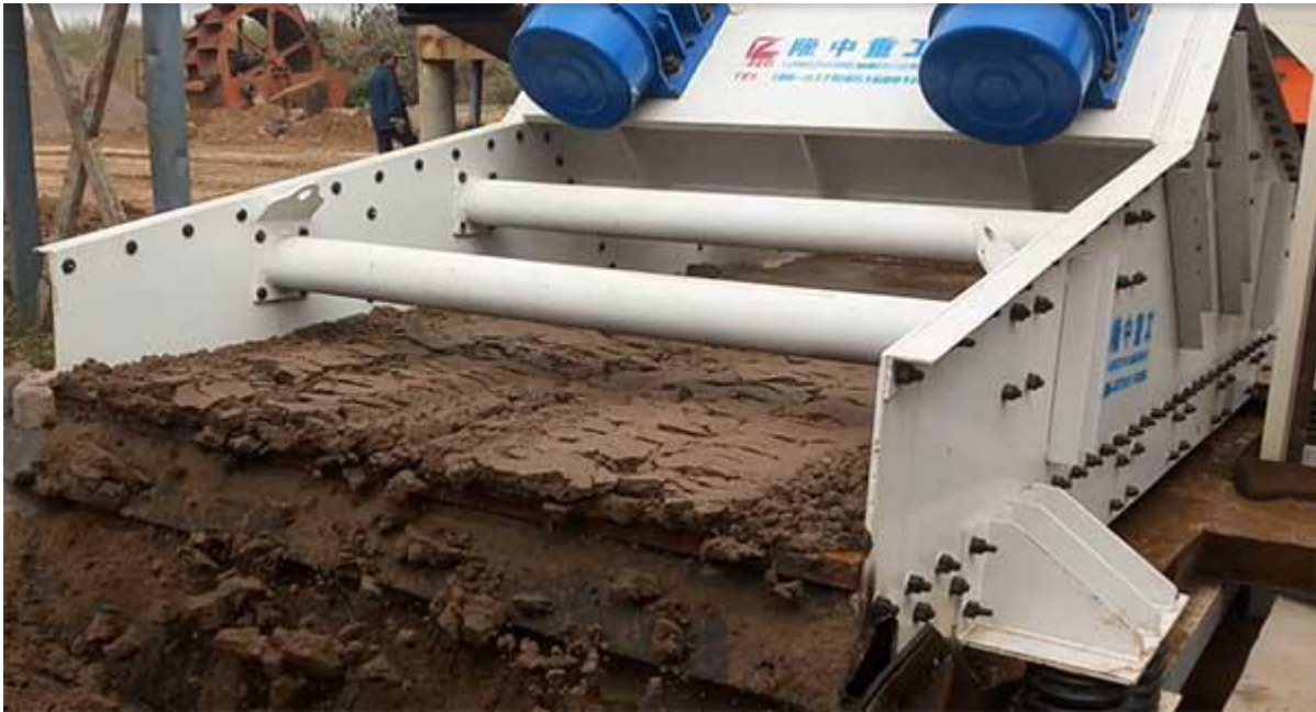
b. Mud water separation muddy water purification from pre-work
