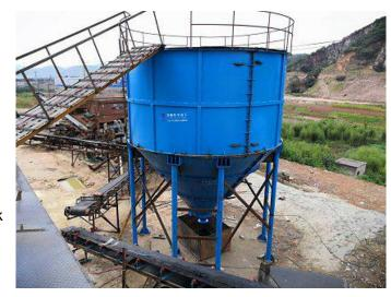
overflow is equipped with filter and baffle, which improve the water quality that poured out.
